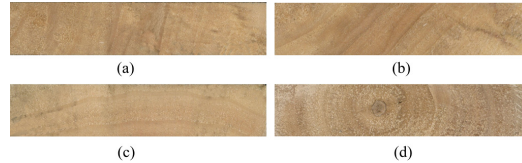
Fig. 2: Typical cross section annual ring orientations (a) group A, (b) group B, (c) group C, and (d) group G.
