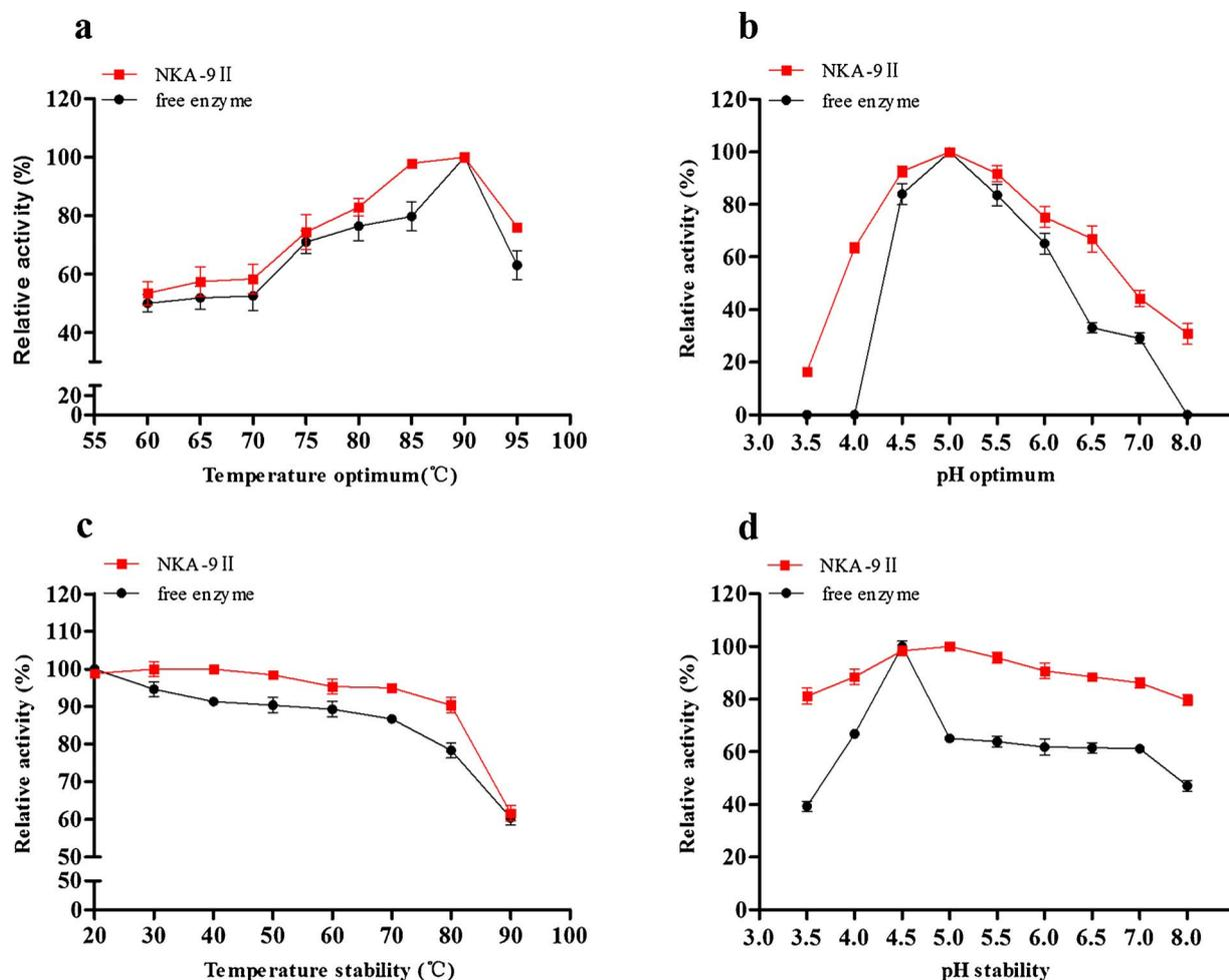
Fig. 3. The properties of free Tpebgl3 and NKA-9II (optimal temperature, optimal pH, temperature stability, and pH stability are shown in panels a, b, c, and d, respectively; the initial activity of NKA-9II at the optimal condition was defined as 100%, and these activities were expressed as relative values).
