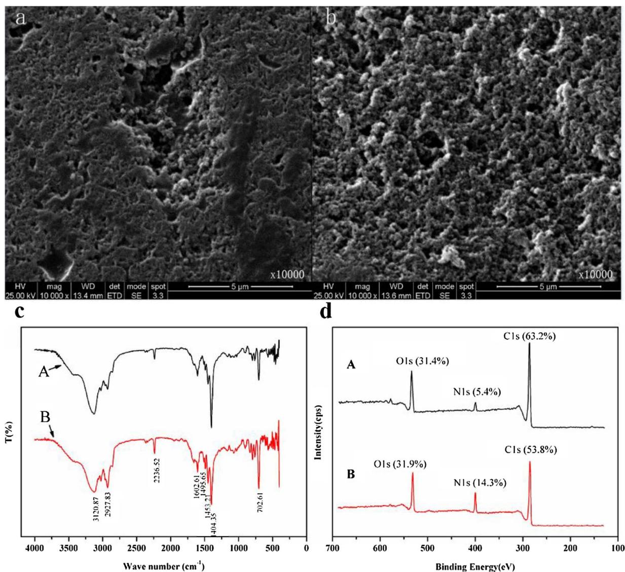
**Fig. 2.** The morphology and structure were characterized by ESEM, FT-IR, and XPS (a: NKA-9 without modification, amplification X10000; b: NKA-9 with 6% PEI treatment, amplification X10000; c: results of FTIR, (A) NKA-9 modified by PEI, (B) NKA-9I, IR KBr ( $\text{cm}^{-1}$ ): 3121 (aliphatic, C–H), 2928 (aromatic, C–H), 2237 (C=C), 1603, 1496, 1453, 1404, 703 (aromatic frame); d: results of XPS, (A) NKA-9 modified by PEI, (B) NKA-9I).
