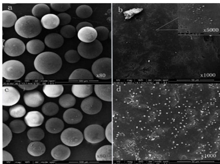
Fig. 4. ESEM of the surface of resin NKA-9II and effect of  $Zn^{2+}$  concentration on the activity of NKA-II (a, b: the surface of NKA-9II in absence of cations c, d: the surface of NKA-9II with metal cation ion  $Zn^{2+}$ ; e: the effect of  $Zn^{2+}$  concentration on the activity of NKA-II; a, c, amplification X80; b, d, amplification X1000).
