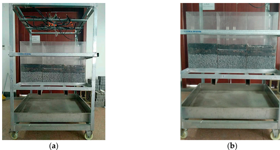
Figure 3. The artificial rainfall system used in this study: (a) The artificial rainfall system with installed model PA pavements; and, (b) Model PA pavements installed in the test rigs.
